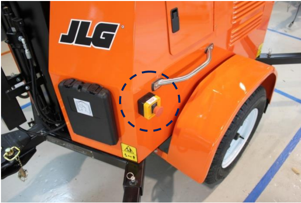
Emergency Stop Button - Circled
