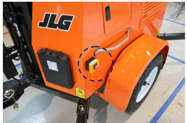
Emergency-Stop Button (circled)
