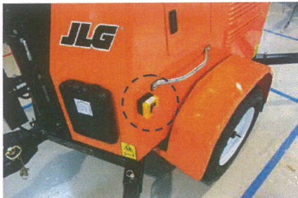
Emergency Stop Button (circled)
