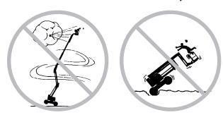
Use extreme care and slow speeds while driving the machine in stowed position across uneven terrain, debris, unstable or slippery surfaces and near holes and drop-offs.
