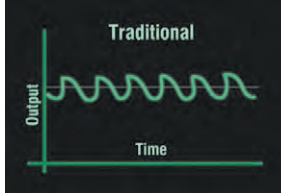
Traditional weld control is more variable around the desired output.
