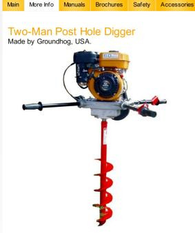
Model Number C715SX Engine Make Subaru Engine 6.0hp EX17D **Engine Features** Over Head Cam, with centrifugal clutch Starting System Recoil Start Fuel Type Petrol Fuel Tank (L) 3.6L Noise Level (dB @ 7m) 66dh Operation Width (mm) Up to 12" Weight (kg) 35kg Manufacturers Warranty 12 months **Engine Warranty** 3 years
