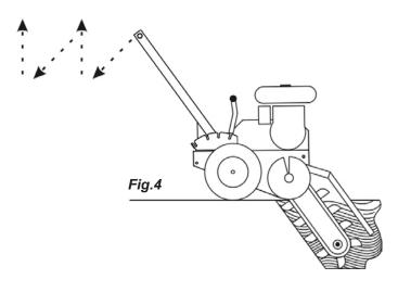
5. Repeat this action until you have finished the job. The wheel lock will aid you in this operation by helping to hold the trencher in position until the next motion is started.
