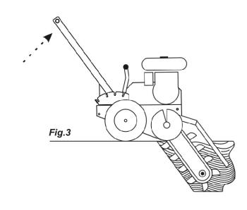
4. Using an intermittent pulling action, pull the trencher toward you 4 to 6 inches then relax your pull, allowing the trencher to again reach the chosen depth. *Fig. 4*
