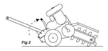
3. Apply downward pressure to the handlebar so the digging chain is not in contact with the ground. Increase the engine speed and hold on to the handlebar with both hands. Slowly relieve the downward pressure on the handlebar allowing the digging chain to penetrate the soil until the chosen depth is reached. *Fig.* 3
