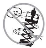
Do not operate the machine in strong or gusty winds. Do not increase the surface area of the platform or the load. Increasing the area exposed to the wind will decrease machine stability.
