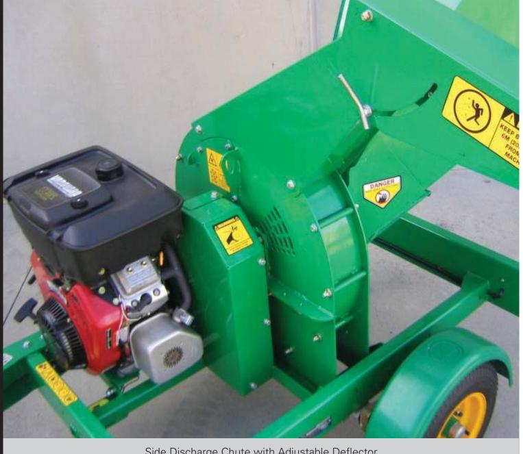
Side Discharge Chute with Adjustable Deflector
