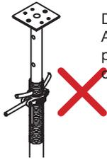
Don't replace an ACROW PROP pin with a piece of reo or a bolt.
