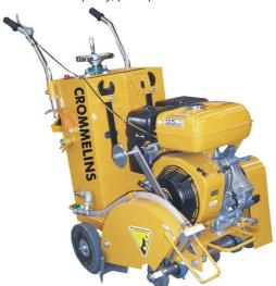
The 14.0hp Floor saw can be fitted with 14" or 16" (355 - 405mm) blades and can cut to a depth of 4.7" (120mm) using a 14" blade or 5.5" (140mm) with a 16" blade.
